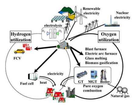
Figure 28 Diagram of utilization of H<sub>2</sub> and by-product O<sub>2</sub> [71]
