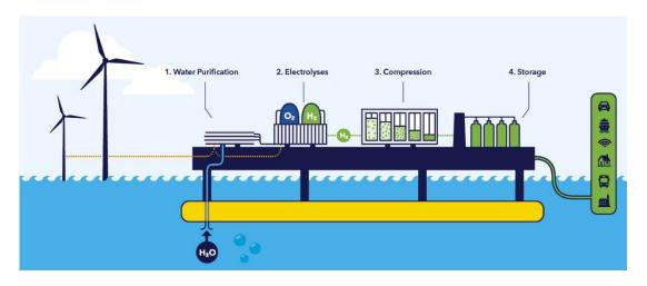
Figure 25 Offshore H<sub>2</sub> plant configuration [59]
