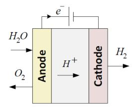
Figure 23 PEM electrolysis process illustration [16]
