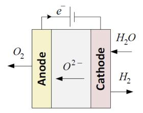
Figure 24 SOE process illustration [16]
