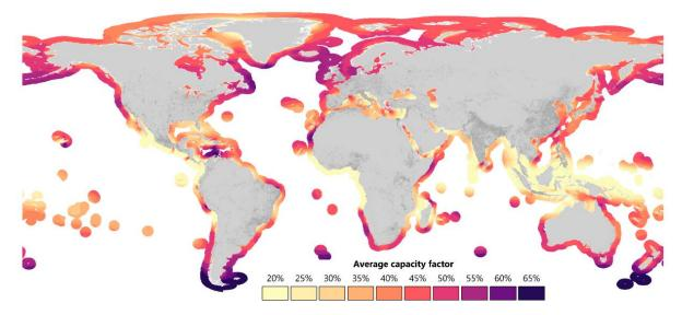
Figure 6 Average simulated capacity factors for offshore wind worldwide [17]
