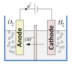
Figure 22 Alkaline electrolysis process illustration [16]
