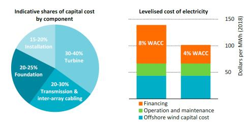
Figure 1 Offshore wind initial investment breakdown by component and LCOE for projects completed in 2018 [17]
