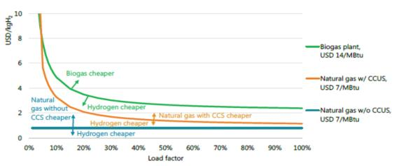
Figure 35 H<sub>2</sub> competitiveness with biogas or natural gas with CCUS [12]
