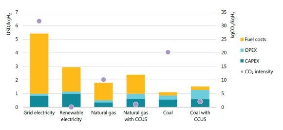
Figure 21 LCOH breakdown and CO<sub>2</sub> intensity for different production pathways2 [12]
