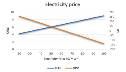
Figure 47 Sensitivity analysis based on electricity price. LCOH and NPV results \*Case 0: Centralised offshore dedicated production
