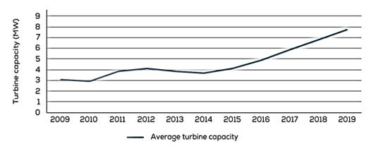
Figure 10 Average capacity per installed turbine [32]
