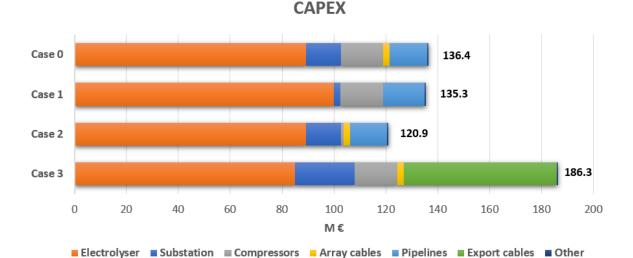
Figure 41 shows the CAPEX breakdown of the different cases.
