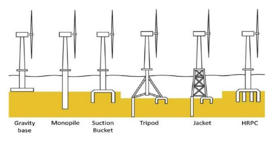
Figure 12 Most common offshore wind turbines structures [22]
